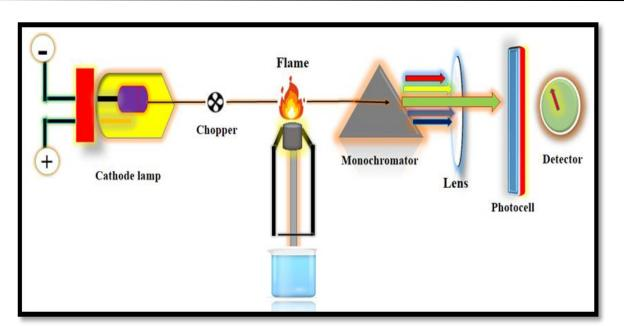
Fig. 3.9. The schematic representation of instrument atomic absorption spectrophotometer.
