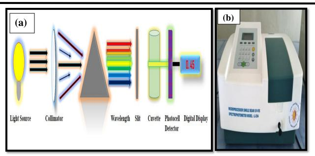
Fig. 3.5. (a) Schematic representation UV- Visible Spectrophotometer (b) Digital UV-Visible Spectrophotometer
