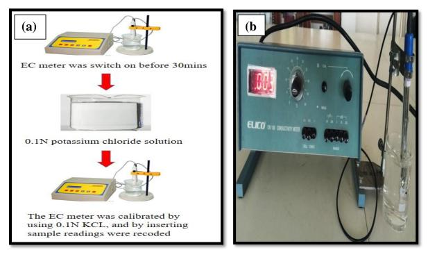
Fig. 3.3. (a) The standard protocol for analysis of electric conductivity and (b) digital electric conductivity meter.
