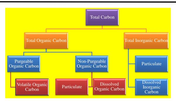
Fig. 3.4. The flow chart represents the types of carbon and its relation.
