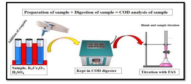
Fig. 3.2. The standard protocol for Chemical Oxygen Demand analysis.
