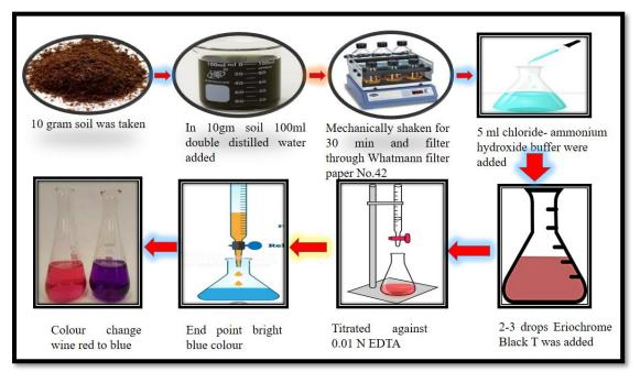
Fig. 3.7. Represents the standard protocol for analysis of calcium.
