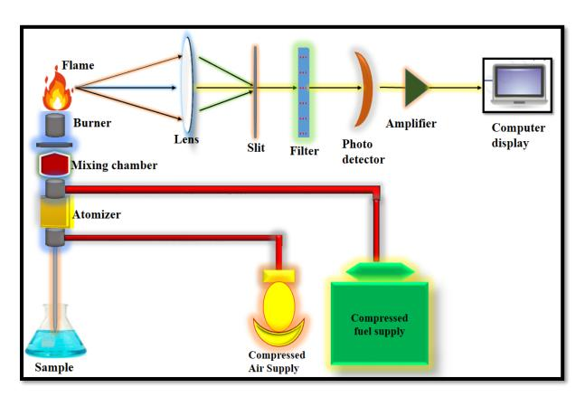
Fig. 3.4. Schematic representation of the Digital Flame Photometer
