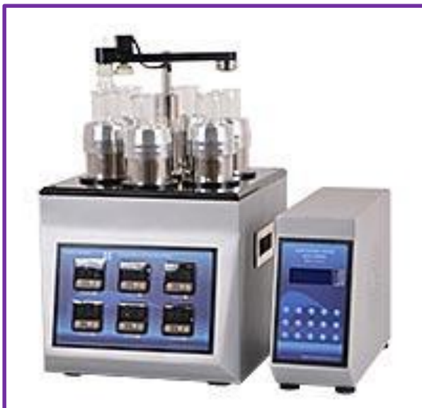
Fig. 2.2 The photograph of SILAR instrument used for thin film deposition [9].
