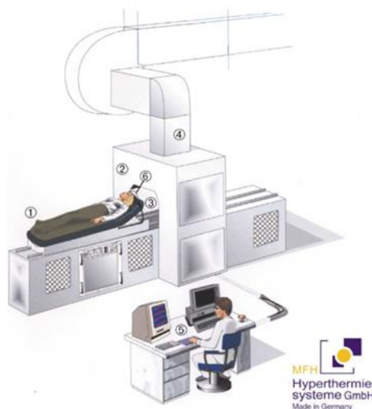
Fig.2.3: Schematic of the first prototype of the Magnetic Fluid Hyperthermia (MFH) therapy System (MFH Hyperthermie systeme GmbH, Berlin, Germany): Highlights include an alternating current magnetic field magnetic field axis that is perpendicular to the patient couch (1), a ferrite-core applicator that operates at 100 kHz (2), an adjustable vertical aperture (3), an air-cooling system (4), and a manual control unit (5). Fluoro-optic probes are used in an intrusive manner to measure temperature [14].
