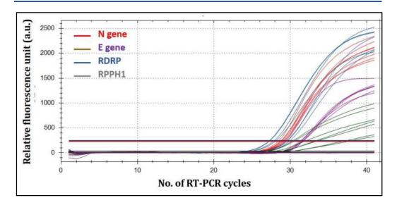
Figure 6.3. RT-PCR of SARS-CoV-2 RNA detection based on glycine@Fe<sub>3</sub>O<sub>4</sub>-RNA conjugate formation (N=6). Highest peak for each gene shows positive control group. Straight lines indicate negative control group.
