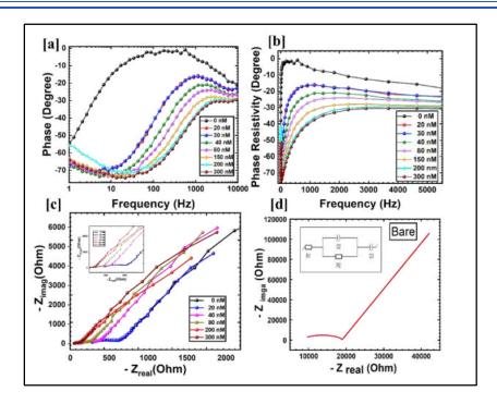
Figure 4.3. Electrochemical impedance spectrometry (EIS) responses of glycine@Fe<sub>3</sub>O<sub>4</sub>-based DNA sensing with DNA concentration range 0 to 300 nM; (a) Bode plot, (b) Phase resistivity spectrum, (c) and (d) Nyquist plots showing significant concentration-dependent DNA separation.
