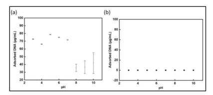
Figure 3.5 Effect of pH by UV-visible DNA quantification on (a) glycine@Fe<sub>3</sub>O<sub>4</sub>-DNA conjugation, and pristine Fe<sub>3</sub>O<sub>4</sub>-DNA conjugation. DNA = 50 µg/mL, temperature = 25°C, nanoparticles = 50 µg/mL, time = 30 min.
