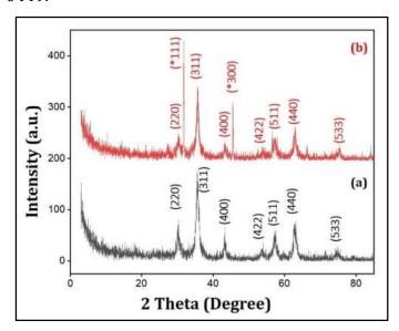
Figure 2.2. X-ray diffractometer (XRD) analysis of synthesized (a) pristine Fe<sub>3</sub>O<sub>4</sub>, and (b) glycine@Fe<sub>3</sub>O<sub>4</sub> nanoparticles.
