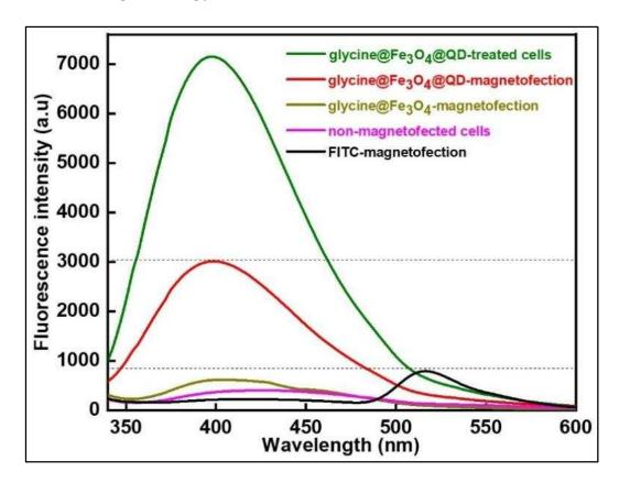
Figure 5.7. Fluorescence spectroscopy to study magnetofection of  $glycine@Fe_3O_4@QD\text{-}DNA$  in MCF-7 cells.
