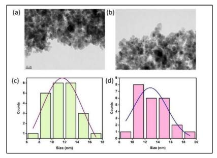
Figure 2.4. Transmission electron microscopy (TEM) photographs at 100kX magnification of (a) pristine Fe<sub>3</sub>O<sub>4</sub>, (b) glycine@Fe<sub>3</sub>O<sub>4</sub> and histograms of (c) pristine Fe<sub>3</sub>O<sub>4</sub>, and (d) glycine@Fe<sub>3</sub>O<sub>4</sub>.
