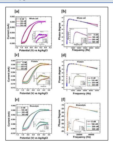
Figure 4.5. Cross reactivity analysis using (a, c, e) cyclic voltammogram, and (b, d, f) EIS responses of glycine@Fe<sub>3</sub>O<sub>4</sub> electrode under the successful addition of whole cell, protein, and bioanalyte with the concentration range from 0 to 300 nM.
