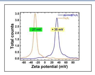
Figure 2.7. Zeta potential analysis of pristine  $Fe_3O_4$  (orange color) shows negative surface charge with the value -27 mV, and glycine@ $Fe_3O_4$  (blue color) shows positive surface charge with the value + 35 mV.
