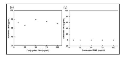
Figure 3.3. Effect of DNA concentration by UV-visible spectroscopy on; (a) glycine@ $Fe_3O_4$ -DNA conjugation, and (b) pristine  $Fe_3O_4$ -DNA conjugation.
