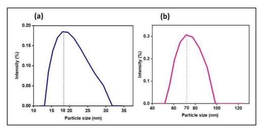
Figure 2.6. DLS analysis of (a) pristine  $Fe_3O_4$ , and (b) glycine@ $Fe_3O_4$  nanoparticles.
