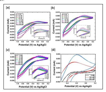
Figure 4.2. Cyclic voltammetry curves of glycine@ $Fe_3O_4$ -modified electrodes with the DNA concentration range from 0 to 300 nM; (a) at 20 mV/s, (b) at 40 mV/s, (c) at 60 mV/s, and (d) the magnified potential window at 20 mV/s showing DNA separation in 1 M PBS electrolyte.
