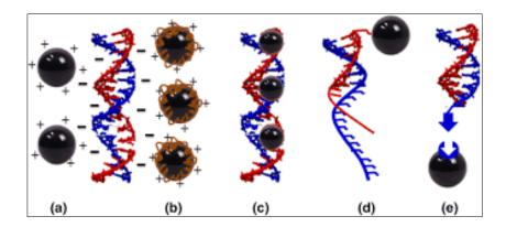
Figure 1.3. Interactions of IONP-NA conjugates; (a) pristine IONP-NA electrochemical interactions, (b) surface functionalized IONP-NA electrochemical interactions, (c) co-precipitation, (d) complementary hydrogen bonding, and (e) targeted nano-covalent interactions [8].
