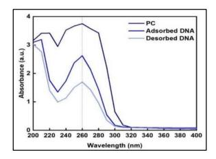
Figure 3.8. UV-visible spectra scan of desorbed DNA from glycine@Fe<sub>3</sub>O<sub>4</sub>. DNA =  $50~\mu g/mL$ , temperature =  $25^{\circ}C$ , glycine@Fe<sub>3</sub>O<sub>4</sub> =  $50~\mu g/mL$ , pH = 7, time = 30~min.
