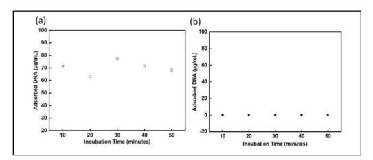
Figure 3.7 Effect of incubation time by UV-visible DNA quantification on; (a) glycine@Fe<sub>3</sub>O<sub>4</sub>-DNA conjugation, and (b) pristine Fe<sub>3</sub>O<sub>4</sub>-DNA conjugation.
