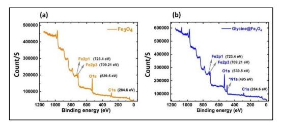
Figure 2.5. XPS analyses of (a) pristine  $Fe_3O_4$  depicting the presence of Fe, O and C in the sample, and (b) glycine@ $Fe_3O_4$  depicting the presence of Fe, O, N and C in the sample.
