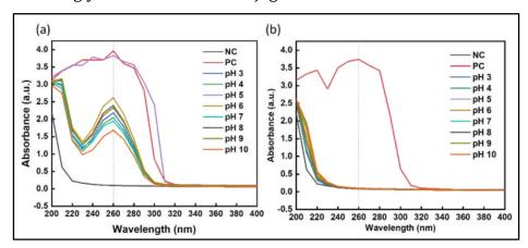
Figure 3.4. Effect of pH by UV-visible spectroscopy on; (a) glycine@ $Fe_3O_4$ -DNA conjugation, and (b) pristine  $Fe_3O_4$ -DNA conjugation.
