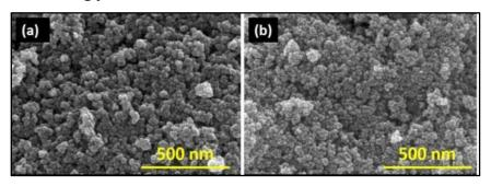
Figure 2.3. Scanning electron microscopy (SEM) photographs of (a) pristine  $Fe_3O_4$  at 30kX magnification, and (b) glycine@ $Fe_3O_4$  at 30kX magnification.
