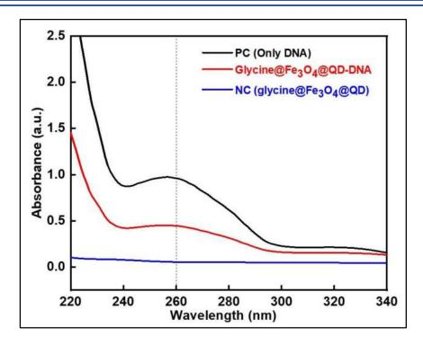
Figure 5.6. UV-visible spectroscopy analysis of glycine@ $Fe_3O_4@QD-DNA$  conjugate formation.
