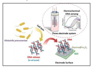
Figure 4.1. Electrochemical *Klebsiella pneumoniae* DNA separation using glycine-modified iron oxide nanoparticles (glycine@Fe<sub>3</sub>O<sub>4</sub>) electrode.
