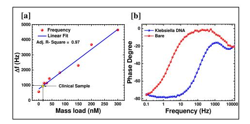
Figure 4.4. Calibration plots for DNA separation; (a) Relationship between DNA mass load and frequency shift provides the R<sup>2</sup> value 0.97, and (b) Bode plot for DNA separation from *Klebsiella pneumoniae clinical* cultures (blue color).
