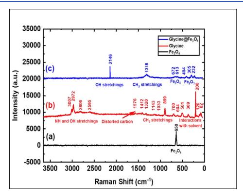
Figure 2.8. Raman spectroscopy analysis of (a) pristine Fe<sub>3</sub>O<sub>4</sub>, (b) pristine glycine, and (c) glycine@Fe<sub>3</sub>O<sub>4</sub>.
