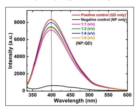
Figure 5.4. Fluorescence spectroscopy analysis for optimization of glycine@Fe<sub>3</sub>O<sub>4</sub>@QD formation.
