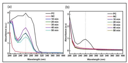
Figure 3.6. Effect of incubation time by UV-visible DNA quantification on (a) glycine@Fe<sub>3</sub>O<sub>4</sub>-DNA conjugation, and pristine Fe<sub>3</sub>O<sub>4</sub>-DNA conjugation.
