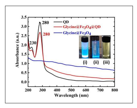
Figure 5.5. UV-visible spectroscopy analysis of glycine@ $Fe_3O_4$ @QD formation; Inset: (i) Only QDs, (ii) glycine@ $Fe_3O_4$ @QD, and (iii) only glycine@ $Fe_3O_4$ .
