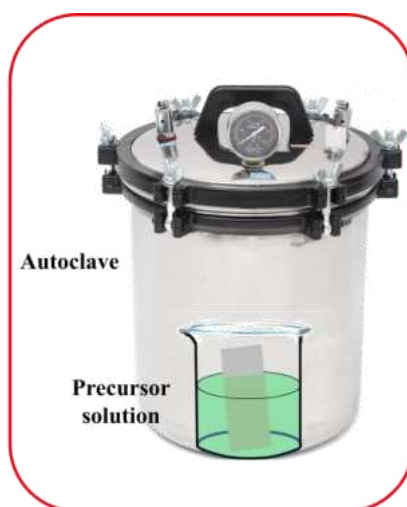
Figure 2.3: Schematic representation of the hydrothermal method.
