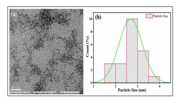
**Figure 3.7:** (a) HR-TEM image (magnification 80KX), and (b) Particle size histogram for PLLCQDs.
