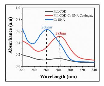
**Figure 4.5:** UV-Vis absorption spectra of PLLCQD-Ct-DNA conjugate showing a red shift in comparison to PLLCQD and Ct-DNA absorption peak.
