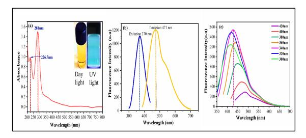
**Figure 3.2:** (a) UV–Vis Spectroscopy, (b) Emission and Excitation spectra, and (c) Emission spectra captured in 20 nm increment in excitation wavelength of PLLCQDs.
