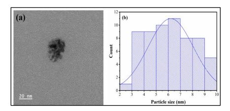
**Figure 5.1:** (a) TEM characterization and (b) particle size histogram of PLLCQD-Ct-DNA conjugate.
