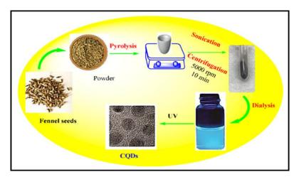
**Figure 1.8:** Schematic representation of fennel seeds CQD synthesis by pyrolysis technique [31].
