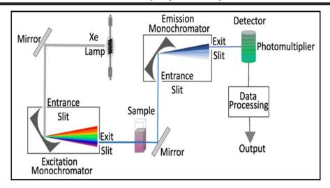
**Figure 2.3:** Schematic diagram of working principle of fluorescence spectroscopy.
