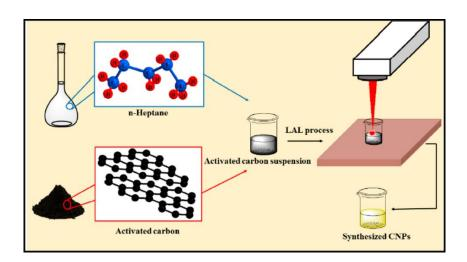
**Figure 1.5:** Schematic representation of laser ablation method for synthesis of carbon nanoparticles [17].
