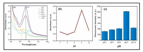
**Figure 4.4:** (a) UV-Vis absorbance spectra of PLLCQD-Ct-DNA conjugate at different pH (2-10), (b) Change in absorbance of PLLCQD-Ct-DNA conjugate at different pH (2-10), and (c) Change in fluorescence intensity of PLLCQD-Ct-DNA conjugate at different pH (2-10).
