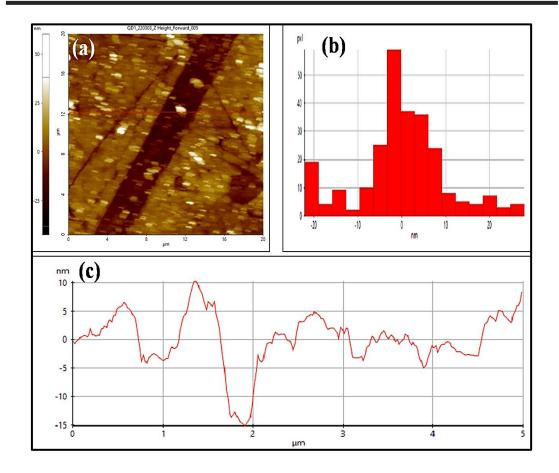
**Figure 3.8:** Atomic Force Microscopy (a) 2D image, (b) Line histogram of particle size, and (c) line graph for PLLCQDs.
