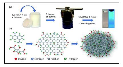
**Figure 1.7:** (a) Schematic representation of CQD by hydrothermal method using 1,5-diaminonaphthalene (1,5-DAN) and citric acid, and (b) Reaction pathway and particle structure [29].
