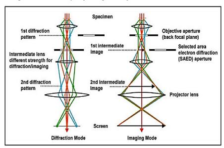
**Figure 2.9:** Diagram showing the principle of the formation of image and diffraction pattern in HRTEM.
