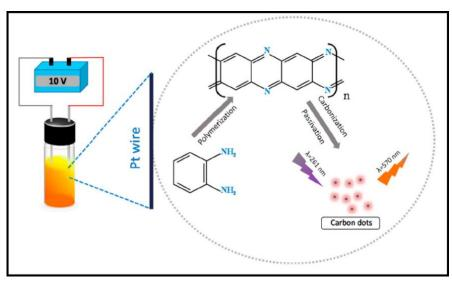
**Figure 1.4:** Schematic representation of CQD fabrication process using the electrochemical method with OPD as the carbon source [15].
