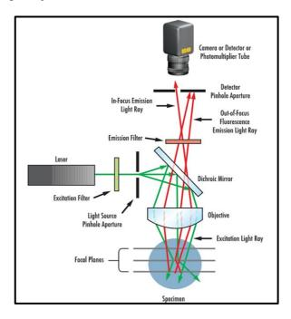
**Figure 2.11:** Schematic presentation of confocal microscopy.
