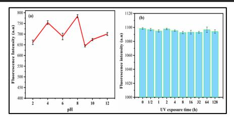
**Figure 3.9:** Relative PL of PLLCQD influenced by (a) pH and (b) exposure time to UV light.
