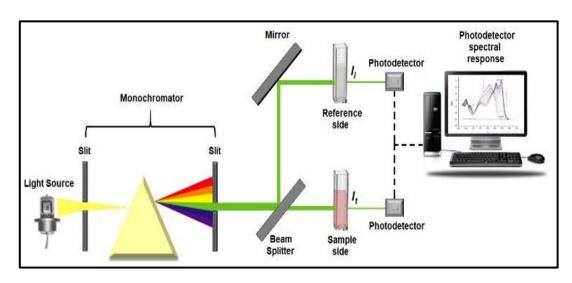
**Figure 2.2:** Schematic representation of working principle of UV-Vis Spectroscopy.
