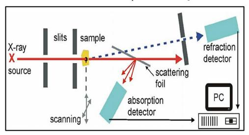
**Figure 2.6:** Diagram showing the working mechanism of XRD.
