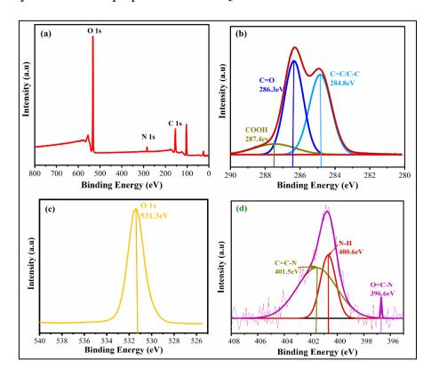
**Figure 3.6:** XPS spectra of PLLCQDs: (a) Survey spectrum, (b) C 1s spectrum, (c) O 1s spectrum, and (d) N 1s spectrum.
