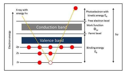
**Figure 2.7:** Schematic representation of working principle of XPS.
