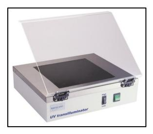
Figure 2.4: UV-transilluminator instrument.
