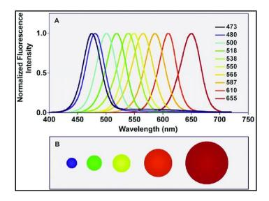
**Figure 1.2:** A) Size-dependent fluorescence emission spectra of QDs and (B) different relative particle sizes with diameters between 2.1-7.5 nm [9].
