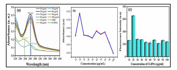
**Figure 4.2:** (a) UV-Vis absorbance spectra showing effect of Ct-DNA concentrations (10-100  $\mu$ g/mL) on PLLCQD-Ct-DNA conjugate, (b) Change in absorbance of PLLCQD-Ct-DNA conjugate at different concentrations of Ct-DNA (10-100  $\mu$ g/mL), and (c) Change in fluorescence intensity of PLLCQD-Ct-DNA conjugate at different concentrations of Ct-DNA (10-100  $\mu$ g/mL).
