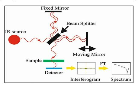
**Figure 2.5:** Schematic representation of FTIR.
