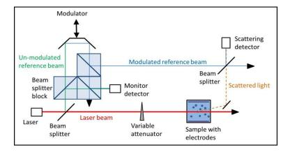
Figure 2.8: Working principle of Zetasizer.
