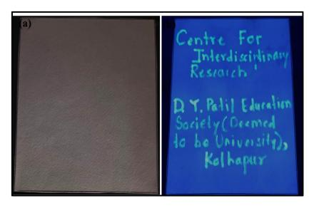
**Figure 3.10:** (a) Text written on a filter paper with PLLCQD ink is invisible in daylight and (b) glows under UV light (365 nm excitation).
