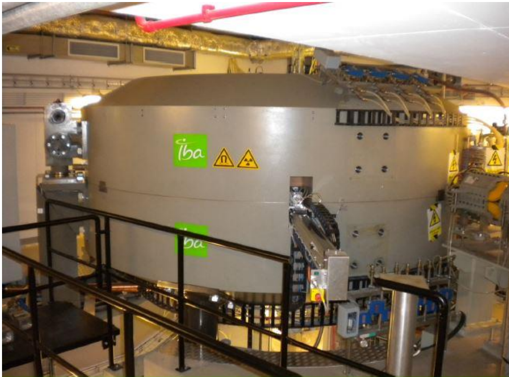
Figure 1.4: The Cyclotron C230 installed at National Hadron Therapy Centre, ACTREC, Tata Memorial Centre, Mumbai.
