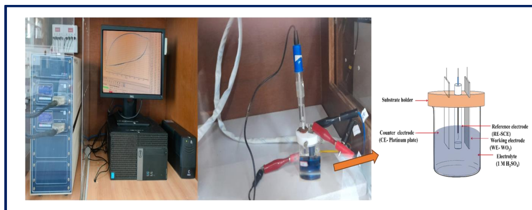
Fig. 3.6 Photograph of electrochemical workstation along with three electrode system.
