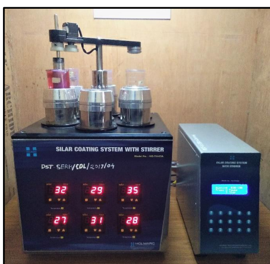
Figure 4.2: The photograph of programmable SILAR coating system used for preparation of rGO-NiWO 4 thin films.
