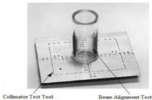
Collimator Test Tool
